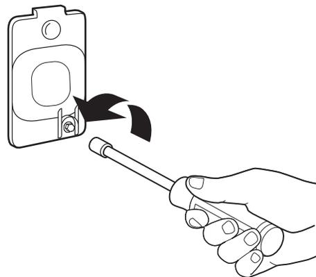
3. Turn bulb counterclockwise. Replace the bulb with a 10 W appliance bulb only. Replace the cover and secure with the screw.
