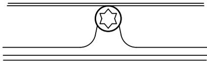
13. Mount the 4<sup>3</sup>/<sub>4</sub>" (12.0 cm) cover box (supplied) to the front of the vent box. Place the keyhole slots over the 2 shoulder screws, align the mounting holes, and secure the cover box to vent box using the 6 screws previously removed from the 1/4" (6.4 mm) deep cover.
