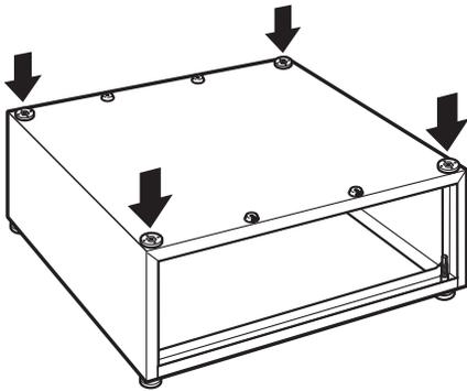
Make sure that all four spacer pads are in place on the top of the pedestal. Spacer pads reduce vibration between the pedestal and the washer/dryer.
