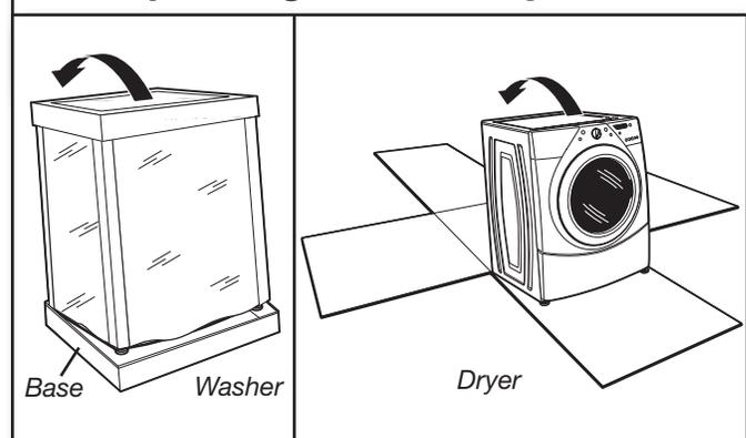
**Washer:** Cut plastic film along dotted cut line around the base. Do not remove the packaging.
