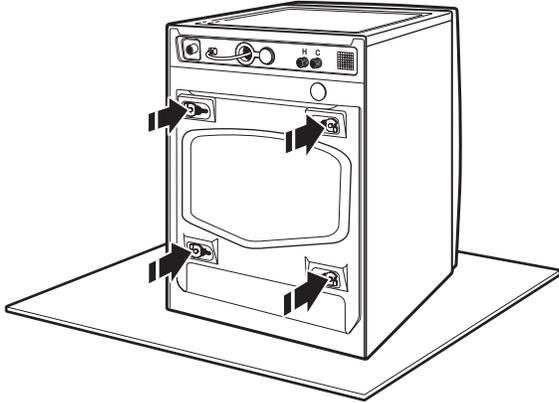
Locate the transport bolts on rear of washer. Transport bolts must remain in washer while pedestal is installed. When laying the washer on its back, hold the base down on the floor. Do not remove the plastic film, corner posts, or top cap.
