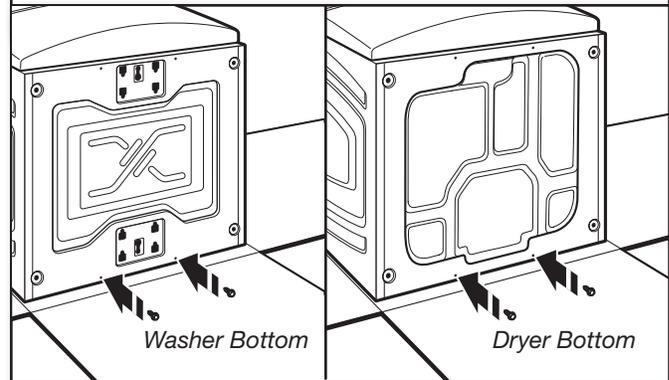
Partially install two of the #12 x 5/8" hex-head sheet metal screws in the lower holes. Leave a space of about 3/8" (10 mm) between the screw head and the bottom of the washer/dryer.
