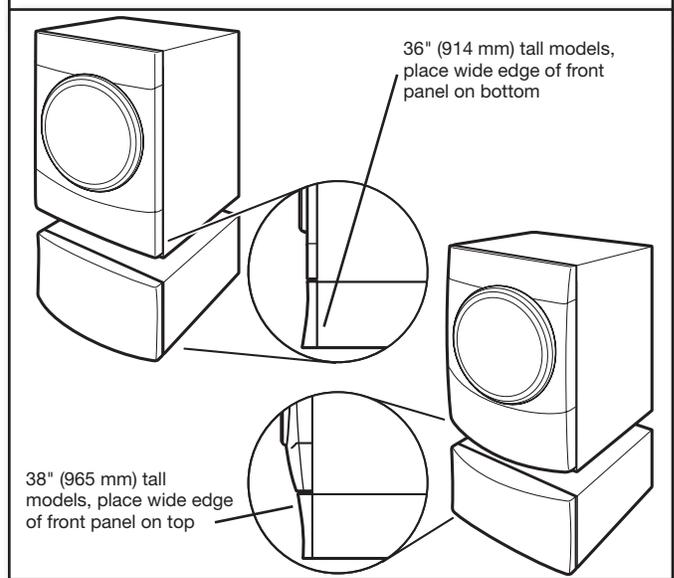
Align the front panel with the pedestal and snap in place.
