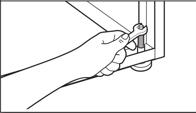
Locate the 1/4" hex-head screws on the top of each pedestal foot. Reach inside the pedestal and use a 1/4" hex-head ratchet or open-end wrench to adjust the feet up or down as needed to level the washer/dryer.
