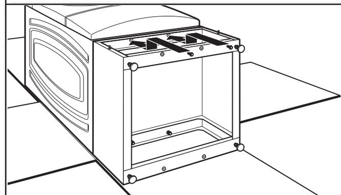
Position the pedestal toward the front of the washer/dryer and install the two remaining hex-head sheet metal screws. Do not tighten completely.
