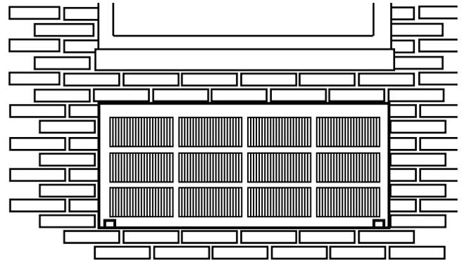
The case is now ready for the installation of the chassis. (For installation of the chassis and appearance front, refer to the instruction packed with the chassis.)
