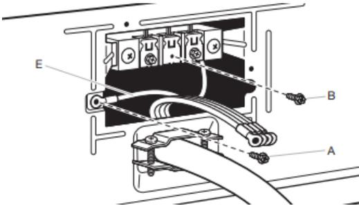
Remove center terminal block screw (B). Remove neutral bond wire (E) from green external ground conductor screw (A).
