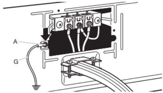
Connect a separate copper ground wire (G) from the green external ground conductor screw (A) to an adequate ground. Insert tab of terminal block cover into slot of dryer rear panel. Secure cover with hold-down screw. Now, go to "Venting Requirements."
