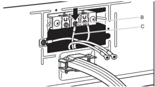
Connect neutral wire (white or center) (C) of power supply cord under center terminal block screw (B). Tighten screw.
