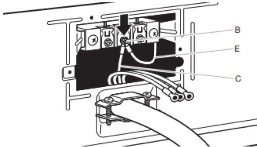
Connect neutral bond wire (E) and neutral wire (white or center) (C) of power supply cord under center terminal block screw (B). Tighten screw.
