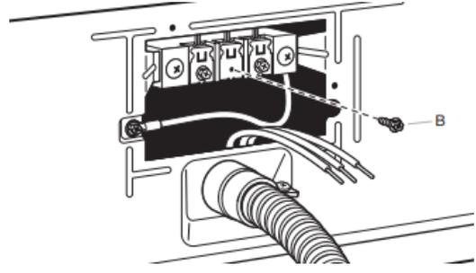
Remove center terminal block screw (B).
