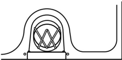
Before installing the vent system, be sure to remove the wire exhaust guard that is located at the exhaust outlet.
