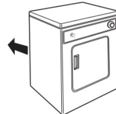
Move dryer to final location. Avoid crushing or kinking the vent. Once the exhaust vent connection is made, remove corner posts and cardboard from under dryer.
