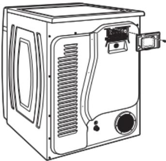
Remove hold-down screw and terminal block cover.
