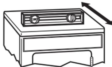
Check levelness of dryer from side to side then from front to back.
