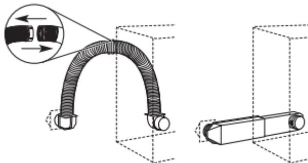
A. Over-the-top installation (also available with one offset elbow)
