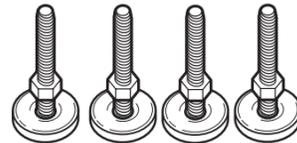
Using a wrench and tape measure, screw leveling legs into leg holes until bottom of foot is approximately 1" (25 mm) to 1 1/2" (38 mm) from bottom of the dryer.
