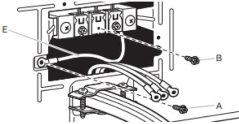
Install the correct strain relief for your electrical connection method. Remove center terminal block screw (B). Remove neutral bond wire (E) from green external ground conductor screw (A).
