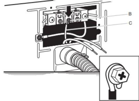
Place hooked end of neutral wire (white or center) (C) of direct wire cable under center terminal block screw (B). Squeeze hooked end together. Tighten screw.
