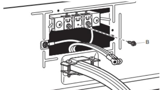
Remove center terminal block screw (B).
