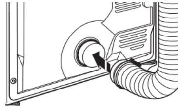
Using a 4" (102 mm) clamp, connect vent to exhaust outlet in dryer. If connecting to existing vent, make sure vent is clean. Dryer vent must fit over dryer exhaust outlet and inside exhaust hood. Check that vent is secured to exhaust hood with a 4" (102 mm) clamp.
