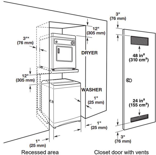
\*Additional spacing recommended. Most installations require a minimum 5 1/2" (140 mm) clearance behind the dryer for the exhaust vent with elbows. See "Venting Requirements."
