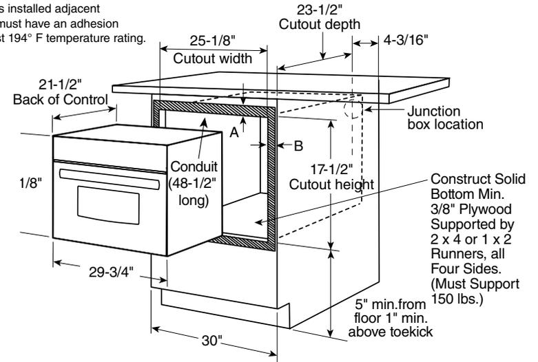
A= Allow 1" overlap of oven over bottom edge of cutout, and allow 1-1/4" overlap at top edge of cutout.
