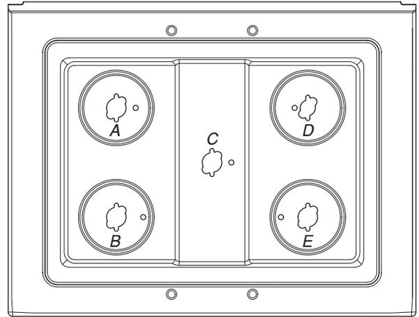
A. Standard burner - Propane gas orifice spud number 088
