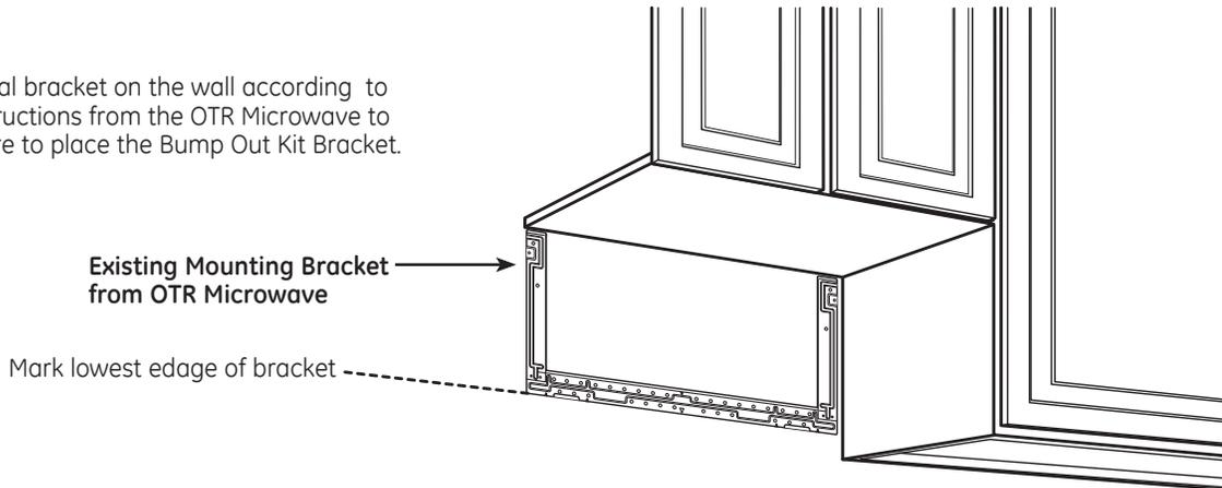
Place the Bump Out Kit Bracket in place of existing bracket location making sure that the bottom edge lines up.
