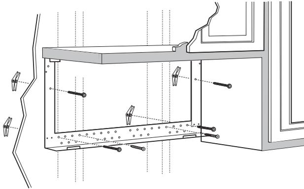
Attach the plate to the wall using (2-4) toggle bolts. At least one wood screw must be used to attach the plate to a wall stud. **NOTE:** Use hardware from OTR packaging.
