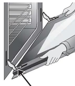
Figure 41: Holding door for removal
