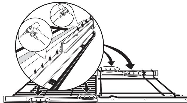
6. Extend and return the glide rack several times along the tracks to distribute the lubrication.
