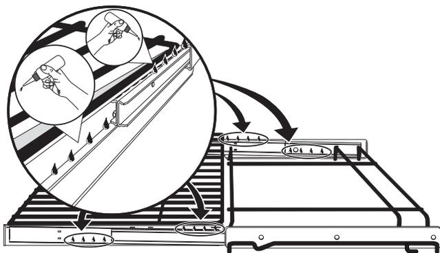
4. Extend and return the glide rack several times along the tracks to distribute the lubrication.
