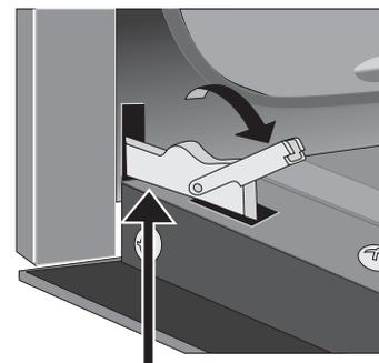
Figure 40: Hinge: unlocked position
