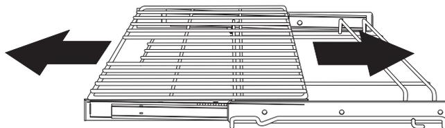
5. Turn glide rack over. Shake graphite lubrication very well before applying. Place four drops of graphite lubrication along the tracks. Repeat on both sides of the glide rack.
