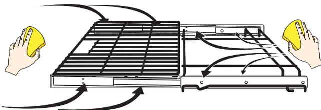
3. Shake graphite lubrication very well before applying. Place four drops of graphite lubrication along the tracks (see area circled on figure below). Repeat on both sides of the glide rack.
