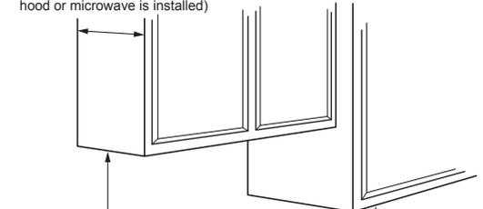
30" MIN. from countertop to unprotected cabinet (when no hood or microwave is installed)
