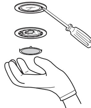
3. Remove the lamp and replace with a 120-volt, 40-watt maximum, halogen lamp made for a G-9 base.
