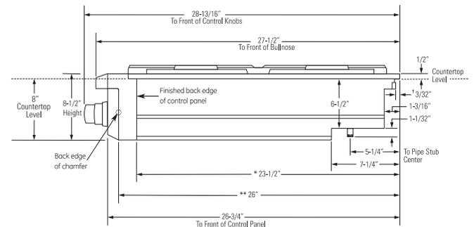
\* Minimum cabinet cutout depth from the back of the rear trim to the back finished edge of the control panel - typically, the minimum cabinet depth front to back. Maximum cabinet cutout depth is 26" minus the countertop overhang.
