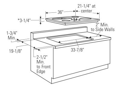
\*3-1/4" deep at the front. 4-5/8" deep at the rear conduit location. Allow 5" minimum clearance below the cooktop bottom to combustible materials.
