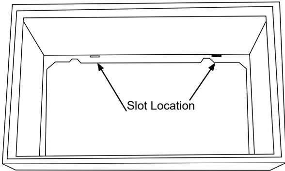
Insert tabs on top of the grille into two slots on the top rear flange. Make sure that both tabs are through the slots and visible inside the case.
