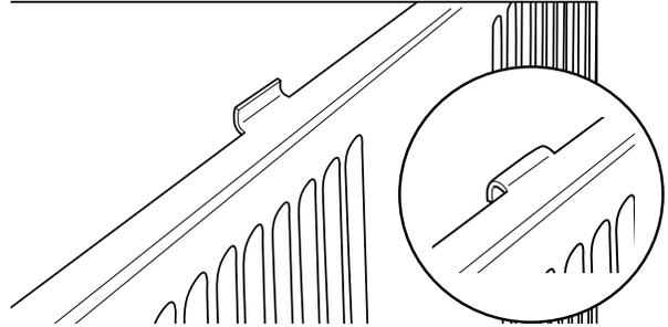
2. Install the "S" clips on the top rear flange of the case approximately 8 inches from each side. Clips fit through the hole in the flange.
