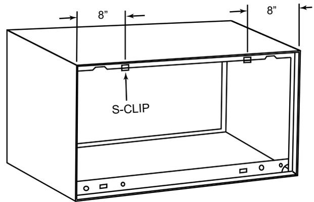
3. Using the ribbon, place the grille completely through the cabinet so that it is outside. Then pull back against the rear of the cabinet and insert the top of the grille up into the clips.
