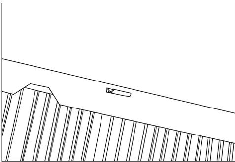
3. Line up the two plastic grommets in the bottom of the grille with holes in the bottom rear flange of the case. Secure with the two included screws from the inside.
