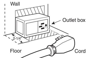
Recommended acceptable electrical outlet area. Orient the electrical receptacle so the length is parallel to the floor.
