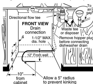
A close-fitting elbow or special shallow sink strainer is necessary to provide clearance between sink drain and dishwasher. Dishwasher furnished with 1/2" I.D. drain hose, 78" long. If using copper tubing, 2" length of 1/2" I.D. rubber hose must be provided to connect copper tubing to pump outlet. Disposer should have 7/8" I.D. dishwasher drain connector.
