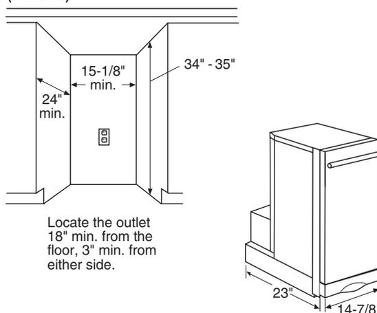
Clearances: Allow 6" clearance to a vertical wall on the right side for bag removal. Allow 23" at the front for a full drawer opening.
