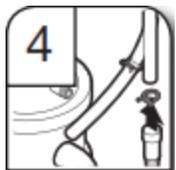
4. Attach drain hose to air gap with large drain hose clamp (provided). Use pliers to squeeze clamp open and move into position. If the drain hose was cut, use a 1 1/2" to 2" (38 mm to 50 mm) screw-type clamp (not provided).
