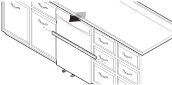
Align front of dishwasher door panel with front of cabinet doors. You may need to adjust alignment to be even with your cabinets.
