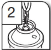
2. Use needle-nose pliers to remove plug.
