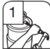
1. Using a hammer and screwdriver, knock plug into disposer.
