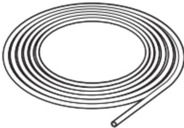
If using copper tubing, measure overall length of copper tubing required to reach the water supply, cut to length, and attach with compression fittings.
