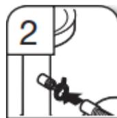
2. Attach rubber end of drain hose to waste tee with a large drain hose clamp (provided). Use pliers to squeeze clamp open and move into position. If the drain hose was cut, use a 1 1/2" to 2" (38 mm to 50 mm) screw-type clamp (not provided).
