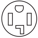
4-wire receptacle (14-30R)
