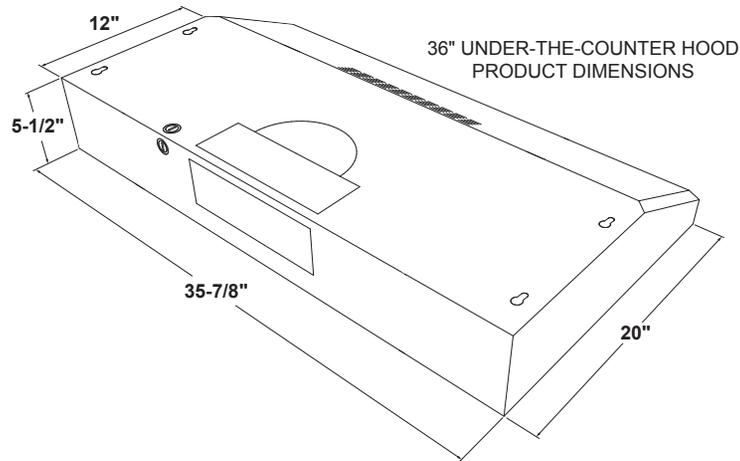
Exhaust outlet connects to 3-1/4" x 10" rectangular duct. Vent top or rear. Includes rectangular damper.
