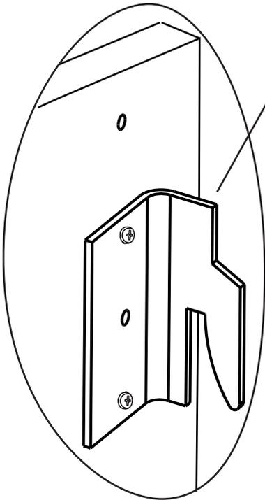
Use lowest set of holes on door and align hook towards outside edge of the door
