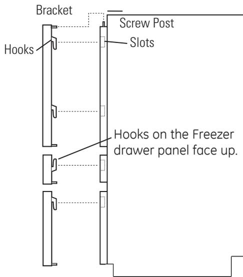
7. Adjust the screw posts up or down under the bracket on top of the door to level the panel.
