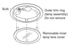
NOTE: Make sure the tabs are inserted into the slots.
