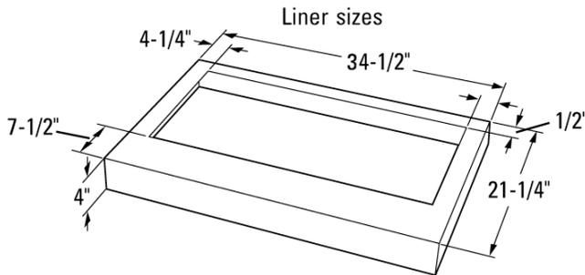
A stainless steel liner is shipped with each hood insert. This non-combustible liner protects the underside of the canopy.
