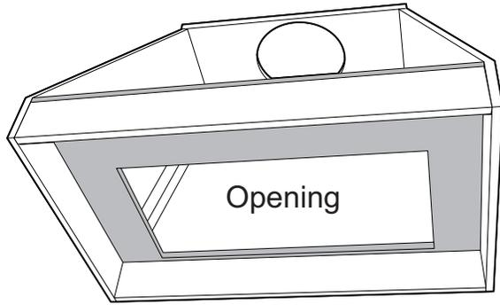
The custom canopy must be sized to fit the insert sleeve. Construct the canopy with an opening that is: 26"W x 13-3/16"D. The opening must be constructed of 3/4" thick material to allow the sleeve locking clips to engage.
