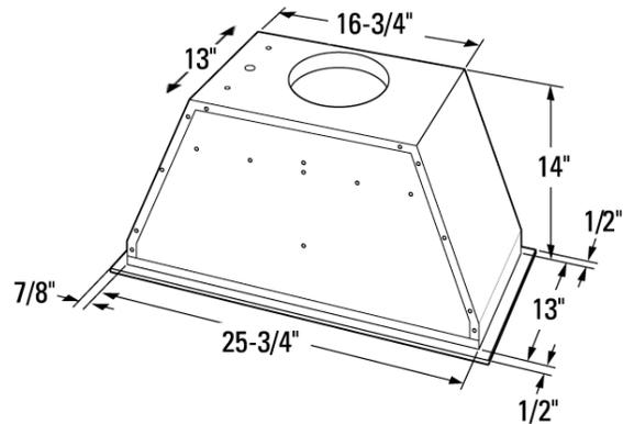
The bottom edge of the insert sleeve has a 7/8" wide flange on the sides and a 1/2" wide flange on the front and back.
