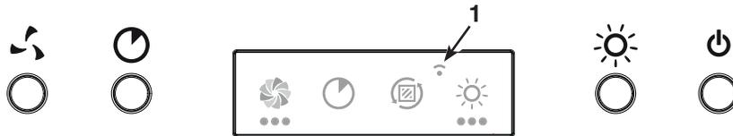
NOTE: At range hood start-up or after a power failure, a small icon (1) appears shortly (for  $\pm 2$  seconds) on LCD screen; this is normal.
