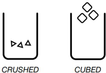
For crushed ice, cubes are crushed before being dispensed. This may cause a slight delay when dispensing crushed ice. Noise from the ice crusher is normal and pieces of ice may vary in size. When changing from crushed to cubed, a few ounces of crushed ice will be dispensed along with the first cubes.
