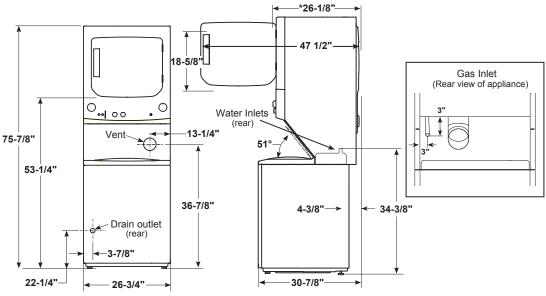
\* Dimension represents door closed including handle and knobs. NOTE: With feet set at mid position, feet can be adjusted +/- 3/8".
