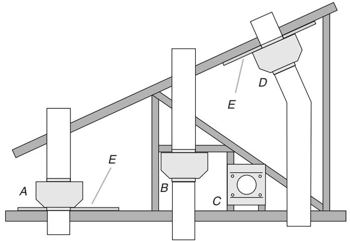
A. Mount on top of ceiling joists.
