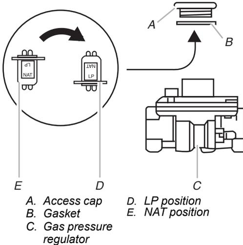
**4. Test the gas pressure regulator and gas supply line.**
