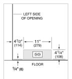
$\ensuremath{\text{NOTE:}}$  The electrical outlet must be positioned with the grounding prong to the right of the thinner blades.
