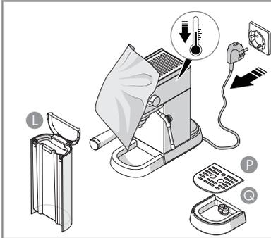
2. Clean the water tank (L), drip tray (Q) and drip grid (P) regularly. Never use caustic or abrasive cleaners, and never immerse the machine in liquid. Do not put components in the dishwasher.
