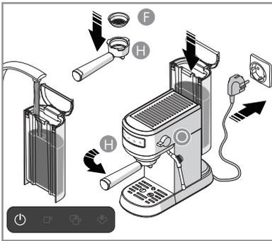
2. Press the power button. The cup buttons blink for up to 40 seconds while the unit warms up.
