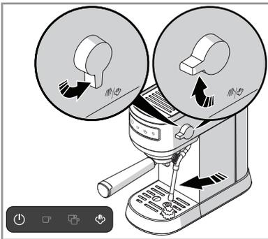
4. Place the pitcher under the steam nozzle and immerse in milk about 1/4" before turning on the knob. Make sure the steam nozzle is positioned so the milk turns in one direction in the pitcher from top to bottom.
