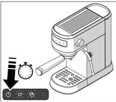
3. Preheating is complete when the buttons stop blinking. Press the Single or Double shot button to start the brewing process.
