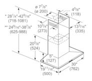
\* Recirculating installation \*\* Ducted installation
