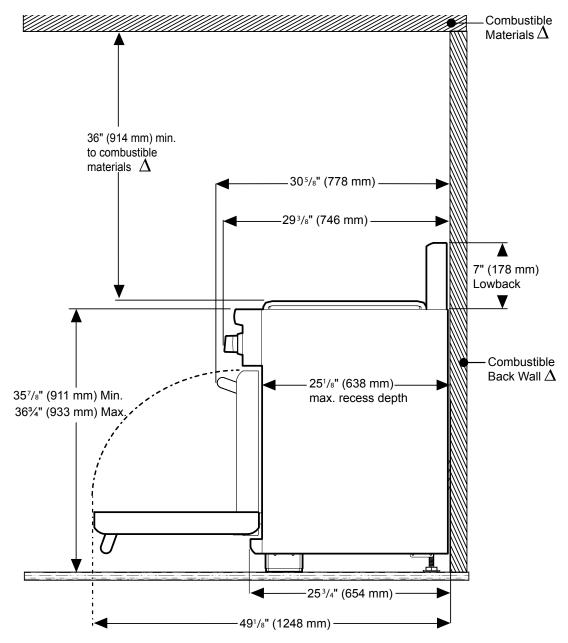
$\Lambda$  As defined in the "National Fuel Gas Code" (ANSI Z223.1, Current Edition). Clearances from non-combustible materials are not part of the ANSI Z21.1 scope and are not certified by CSA. Clearances of less than 6" (152 mm) must be approved by the local codes and/or by the local authority having jurisdiction.
