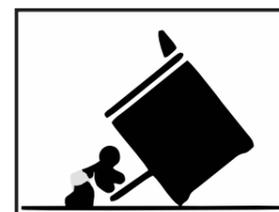
To reduce the risk of tipping the range, the range must be secured by a properly installed **Anti Tip device**. **AFTER THE RANGE HAS BEEN INSTALLED, CONFIRM THAT THE ANTI-TIP DEVICE HAS BEEN PROPERLY INSTALLED AND VERIFY THAT THE ANTI TIP DEVICE IS PROPERLY ENGAGED.** Refer to the installation manual for instructions.
