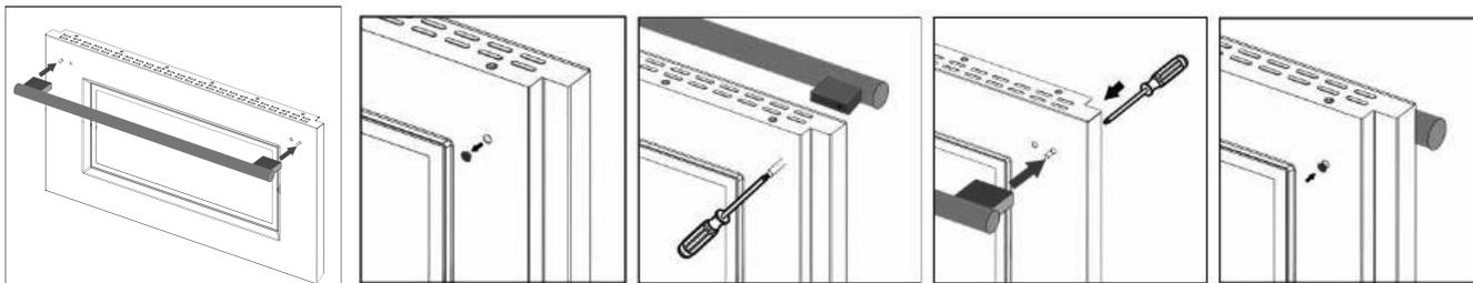
1. Remove the black rubber cap on the inside of oven door. (Do not throw it away).
