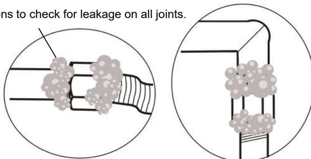
**▲WARNING DO NOT use a flame to check for gas leaks!**
