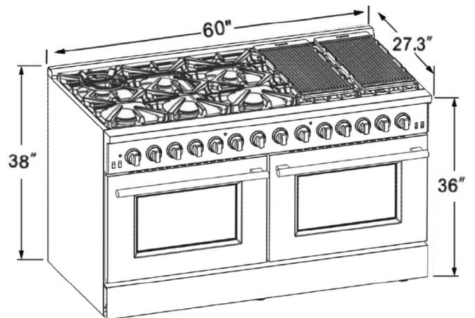
This range may be installed directly adjacent to existing countertop-height cabinets (36" or 91.5 cm from the floor). To achieve the best look, the cooktop should be level with the cabinet countertop. This can be accomplished by raising the unit using the adjustment spindles on the legs.
