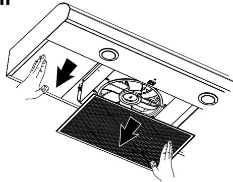
Remove the grease filter and the left side panel
