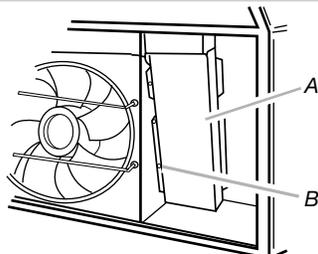
3. Remove the power supply knockout from the top or rear of the vent hood (depending on the incoming location of your home power supply cable) and install a UL listed or CSA approved 1/2" strain relief.
