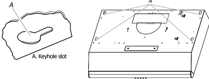
2. Use 1/8" (3 mm) drill bit and drill 4 pilot holes as shown. NOTE: Make the drill holes on the thin area of the slot.
