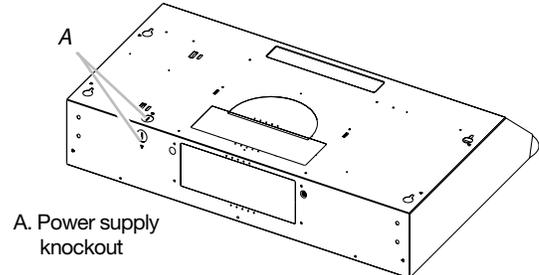
4. Using 2 or more people, lift the hood into final position. Feed enough electrical wire through the 1/2" UL listed or CSA approved strain relief to make connections in the terminal box. Tighten the strain relief screws.
