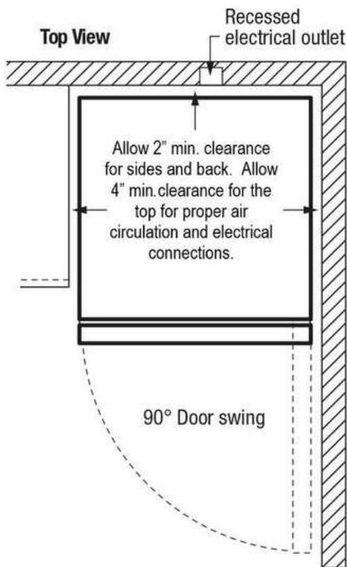
\* When installing refrigerator adjacent to wall, cabinet or other appliance that extends beyond front edge of unit, 20" minimum clearance recommended to allow for optimum 140° door swing.
