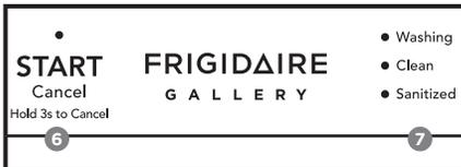
6. **START/Cancel** starts or cancels a cycle. To start the cycle, press START/Cancel button and immediately close the dishwasher door. To cancel the cycle, open the dishwasher door, then press and hold the START/Cancel button for 3 seconds until the cycle and option LEDs turn off.
