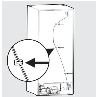
12. Grasp the other end of the plastic tube, and firmly push it into the quick connection on the valve until it bottoms out.
