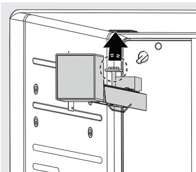
10. Connect the wiring harness to the water valve, making sure the connection is tight, and then install the mounting box and box cover on the plug.
