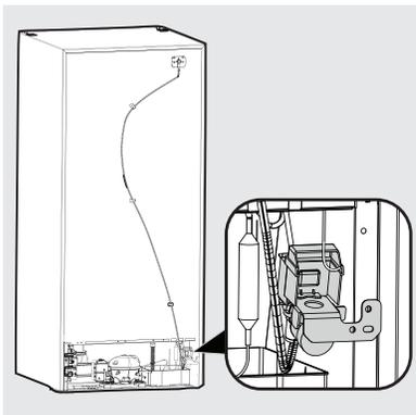
13. Clean the back of the cabinet with a commercial household cleaner, ammonia, or alcohol before applying the clamps. Secure the plastic water supply tubing to the back of the cabinet with three plastic clamps.
