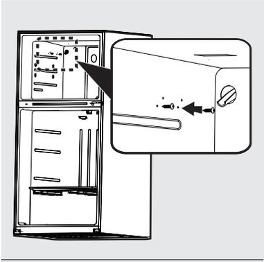
8. Mount the ice maker onto the two ice maker mounting screws you installed in step 5. Make sure the water inlet tube is sitting inside the fill cup and the ice maker is level, and then tighten the screws.
