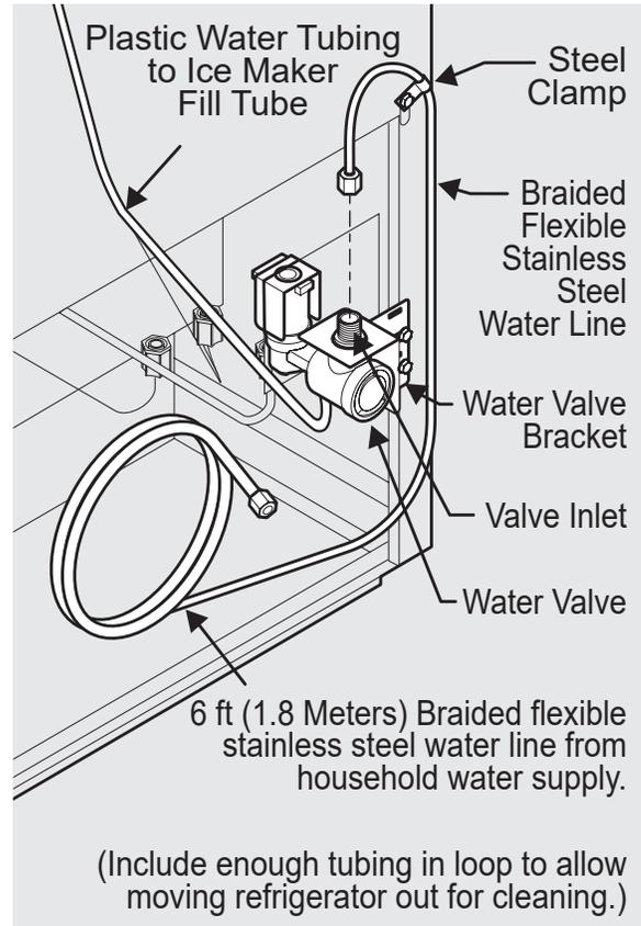
6. With the steel clamp and the screw, secure the water supply line to the rear panel of the refrigerator as shown.
