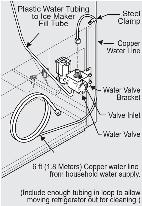
5. Secure the copper line to the clamp (as shown), using the existing screw.
