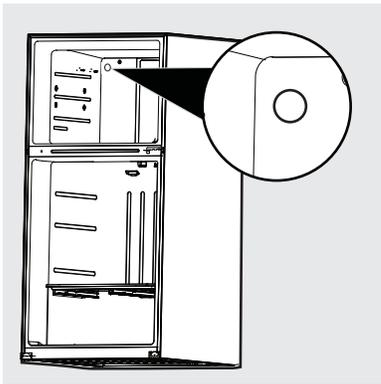
2. Remove the label covering the ice maker hole on the back of the unit, and then remove the foam from inside the hole using needle nose pliers. Keep the foam for future use. See Figure 2.
