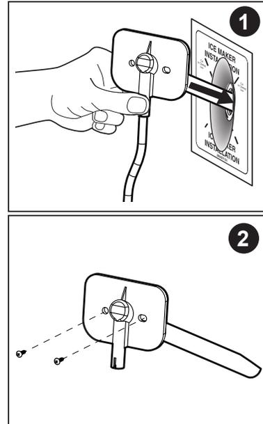
4. While squeezing the tube clamp, slide the clamp over the full tube. While still squeezing the clamp, insert one end of the plastic tube into the fill tube as far as it will go, and then slide the clamp down to keep the fill tube in place. Push the plastic tube in as far as it will go, and put the tube clamp in place over the fill tube to avoid leaks.
