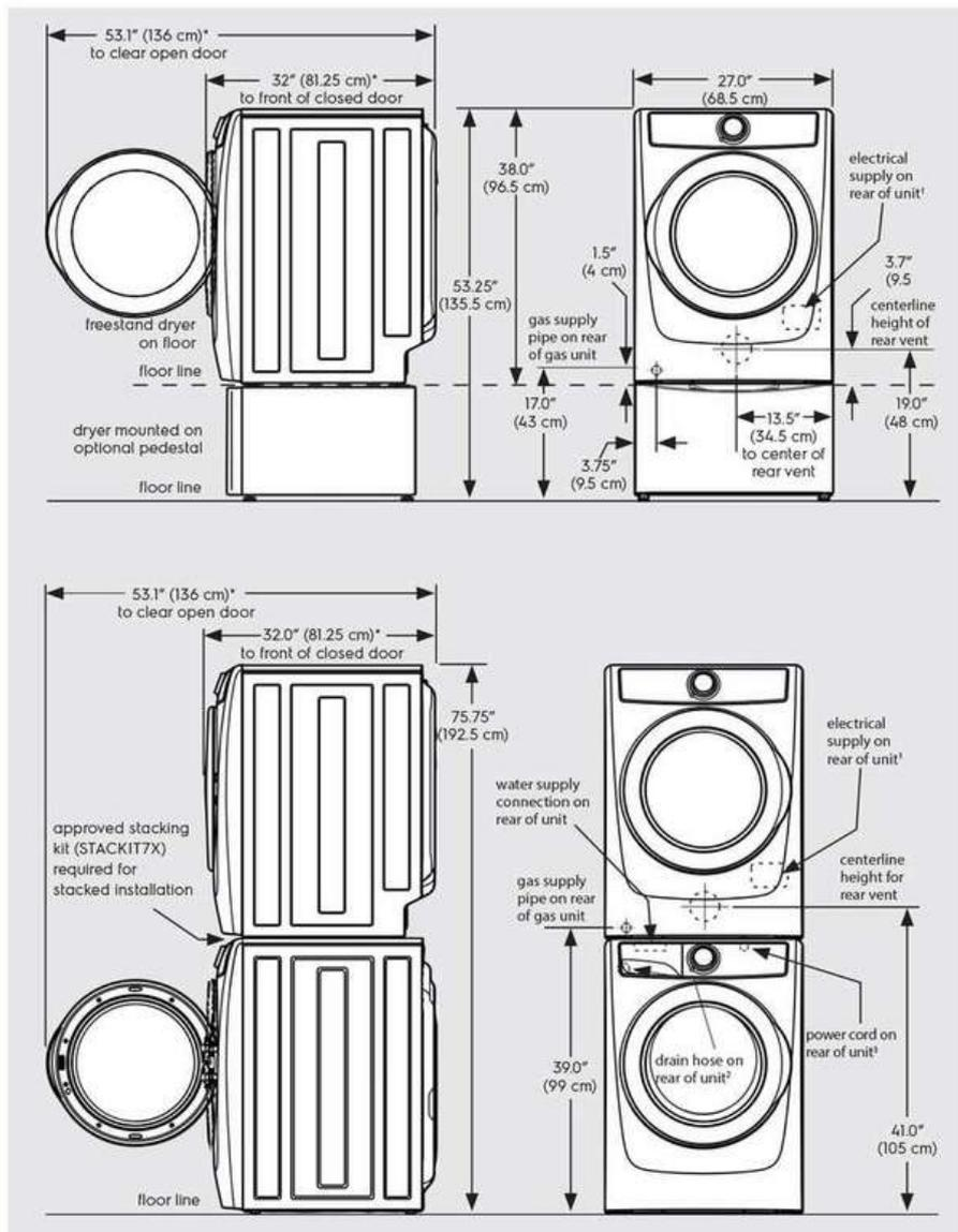
\* Connection of water inlet hose on steam dryer adds 3/4 in. (2 cm) to installation depth.
