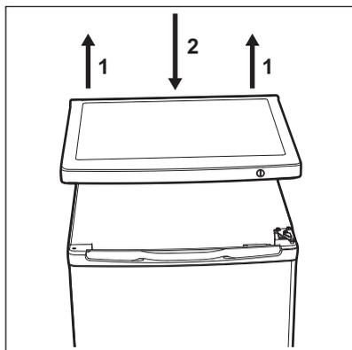
3. Unscrew top hinge. Remove the lid and place it on a soft pad to avoid scratching.
