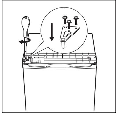
8. Place top cover on the back and fix with 2 screws.
