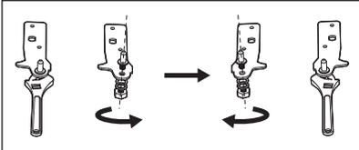
6. Re-fit the bracket fitting the bottom hinge pin. Replace both adjustable feet.
