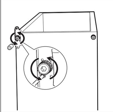
7. Re-place the door. Align it horizontally and vertically so the seals are closed on all sides. Tighten the top hinge.
