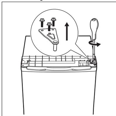
4. Unscrew bottom hinge. Remove adjustable feet from both sides.
