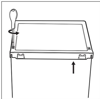
2. Remove the top cover and thermostat knob. Place it aside.
