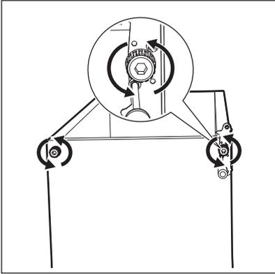
5. Unscrew and remove bottom hinge pin, turn the bracket over, and replace it.
