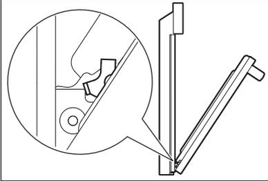
4. Pull the bottom of the door toward you while rotating the top of the door toward the appliance to completely disengage the hinge levers.
