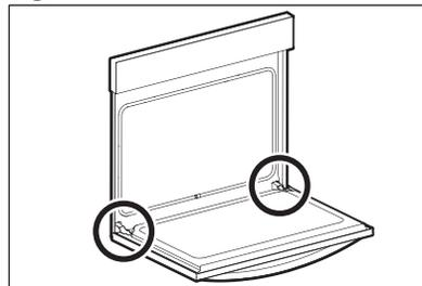
2. Pull up the lock located on each hinge support toward front of the oven until the lock stops. You may have to apply a little upward pressure on the lock to pull it up.
