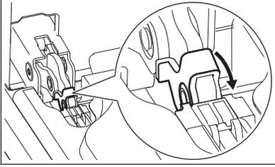
3. Grasp the door by the sides, and close the door until the door frame makes contact with the unlocked hinges.
