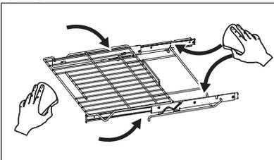
3. Shake graphite lubrication very well before applying. Apply to loading guides, and rotation pin. Repeat on both sides of the glide rack.
