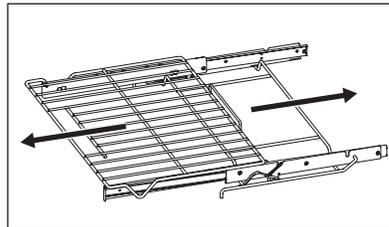
5. Turn the rack upside down and apply graphite lubrication to the insides of the loading guides.
