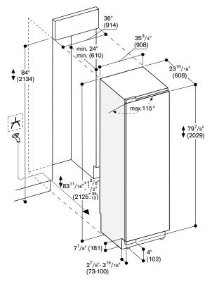
The door face dimensions are designed for a maximum gap of ½" (3 mm). See more details on page 252.
