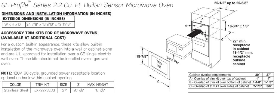
NOTE: Allow an additional inch of clearance beyond trim kit frame on all sides to prevent the trim kit from blocking any outside adjoining cabinets/obstructions. Reference below drawing.
