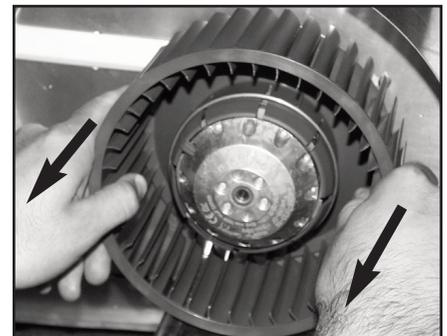
Install 4 screws into the location shown below. Do not tighten screws down fully, leave a 1/8" gap. Hang blower unit onto blower plate (screws through the large part of the keyholes. Slide the blower to its position (screws in the small part of the keyhole). Tighten the screws.
