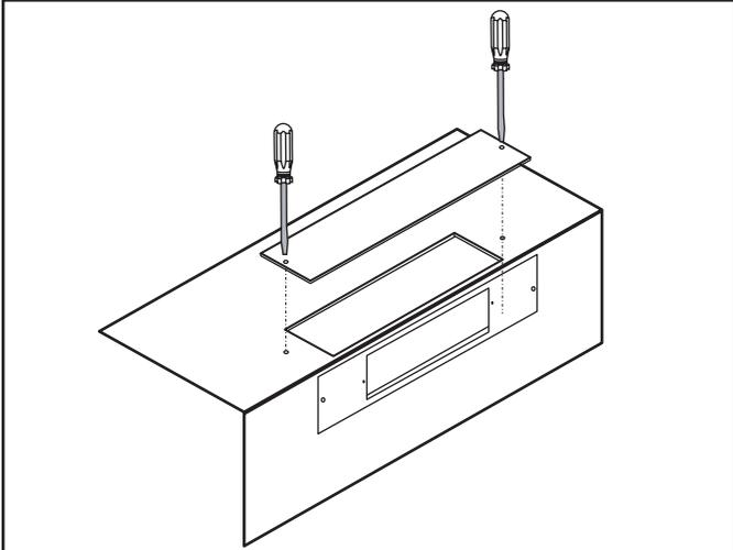
When a vertical discharge has been chosen, discard the damper mounting plate from the back of the hood and install the block off plate from the previous step in its place.
