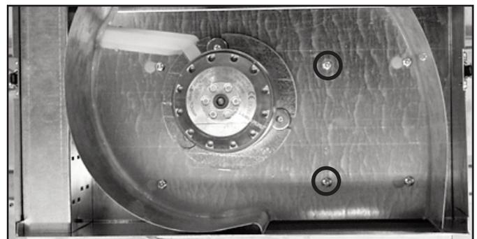
Align damper screw holes with holes in hood to properly position the damper on hood. Using two (2) standard 1/2" screws (1 per side), secure the adapter to the top (or back) of the hood. Seal the adapter to the hood using duct tape.
