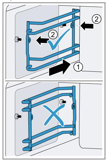
The shelf supports for the left and right side of the cooking compartment are different.
