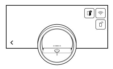
On the left-hand side, the display shows the symbols and texts with information on the current status of the appliance. On the right-hand side, the display shows the touch fields of the control center.
