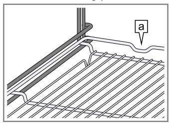
**Note:** To completely pull out the wire rack, lift it up slightly and pull it out with both hands.
