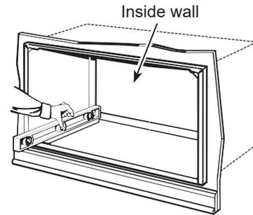
2. Firmly secure the wall sleeve to the wall structure by drilling holes in the appropriate location. Do NOT drill any holes in **the bottom of the wall sleeve**. Use appropriate screws, lag bolts, etc. to attach the wall sleeve to the wall structure.
