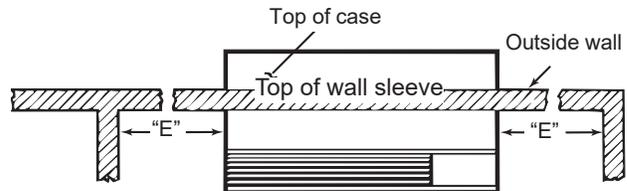
**NOTE: If an internal drain is to be used, install the wall sleeve level from side to side and level from front to rear.**
