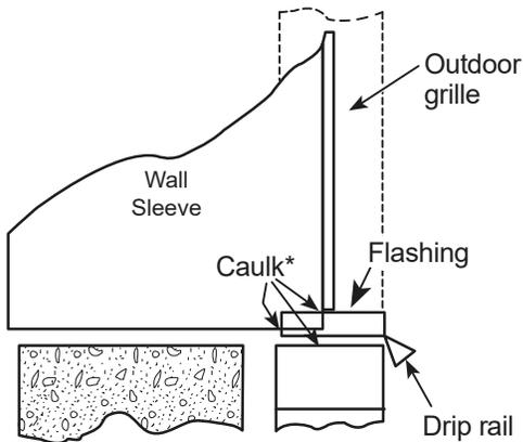
**\*NOTE:** It is critical to caulk around perimeter of wall sleeve on all four sides where it joins the building to prevent air and water infiltration.
