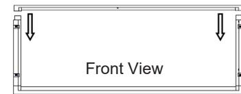
5. (If required) Locate weather barrier and attach to the rear of the assembled sleeve with four (4) supplied white push pins.
