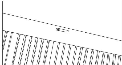
3. Line up the two plastic grommets in the bottom of the grille with holes in the bottom rear flange of the . Secure with the two included screws from the inside.
