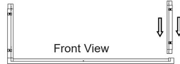
4. Locate top panel and align with top of right and left side panels. Fully insert top panel into right and left side panels until locking tabs lock completely.
