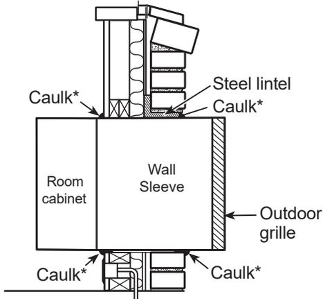
**\*NOTE:** It is critical to caulk around the perimeter of the wall sleeve on all four sides and on the outside and the roomside where it joins the building to prevent air and water infiltration.
