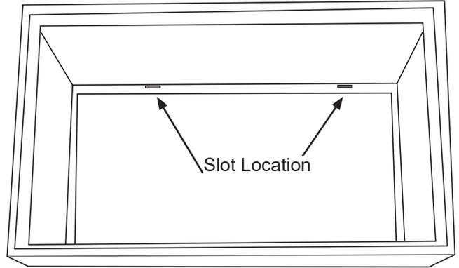
Insert tabs on top of the grille into two slots on the top rear flange. Make sure that both tabs are through the slots and visible inside the .
