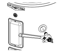
**NOTE:** The segmented anode will be installed in the side port where the original T&P was previously installed.
