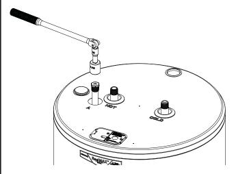
Remove anode rod by lifting straight up (once fully loosened). Needle-nose pliers may be needed to help pull up a few inches from foam hole.
