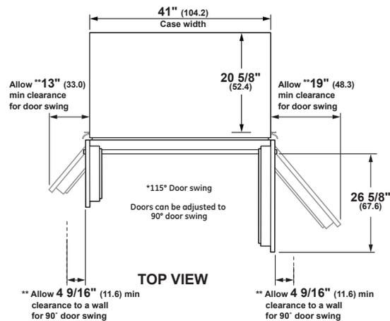
\*\* These refrigerators are equipped with a 3-position door stop. The factory-set 115° door swing can be adjusted to 90° if clearances to adjacent cabinets or walls is restricted. Allow a 15" minimum clearance to wall for pan removal. If the 90° door stop position is used, pan access is maintained, but pan removal is restricted. A 130° door swing option is available for standard installation only. Dimensions based on custom handle height of 2 9/16" (6.5).
