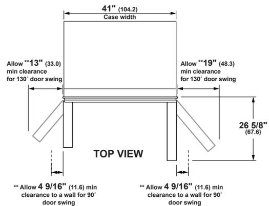
\*\* These refrigerators are equipped with a 3-position door stop. The factory-set 115° door swing can be adjusted to 90° if clearances to adjacent cabinets or walls is restricted. Allow full 130° door swings for pan removal. If the 90° door stop position is used, pan access is maintained, but pan removal is restricted. Dimensions based on custom handle height of 2 9/16" (6.5).
