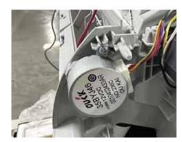
The motor moves the louver side to side depending upon selections made at the remote control.
