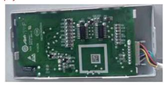
The indoor display has an infrared communication circuit that receives operating commands from the remote control. This display will indicate operating modes, error codes, indoor air temperature, timer status, and power status.
