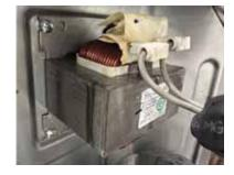
The Reactor is a power filter. It is unlikely to ever have an electrical failure of this component.
