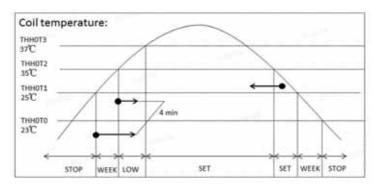
The indoor fan is controlled based on the coil temperature, as shown in the figure above.
