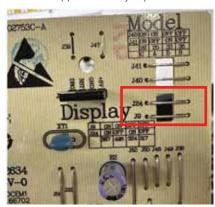
$\rm J40$  and J41 Selects EEPROM codes A, B, C and D. Cut wires to match the model type listed below:
