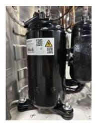
The Accumulator is located in the suction line circuit at the entrance to the compressor. The accumulator helps prevent liquid refrigerant from entering the compressor during run operation.
