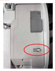
If the remote control is non-functional, the Emergency Button can be used.  $73-78^{\circ}F$  will be maintained, until commands are received via the remote control.
