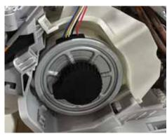
The Fan Motor is a variable speed motor. Fan speed will vary depending upon the temperature variation from set point, or can be set with the remote control to maintain a single set speed.
