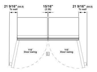
\*\*Dimensions based on handle height of 2 9/16" (6.5) and a hand clearance of 2" (5.1).
