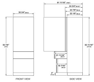
\*Depth dimension without handle. Statement handle adds 2 9/16" depth. Minimalist handle adds 2 1/8" depth. \*\*Includes 3/4" door panel
