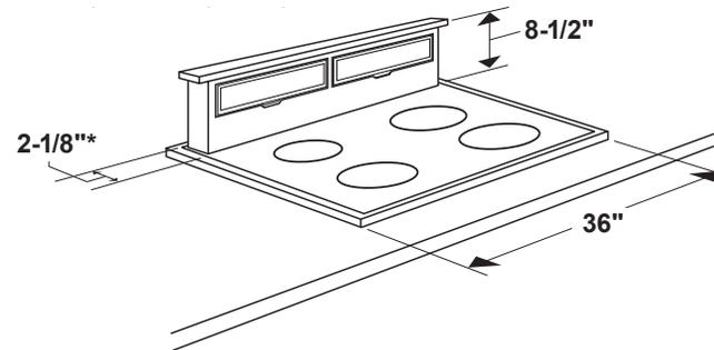
\*Minimum distance required between the back edge of the cooktop and the back of the cutout in the countertop
