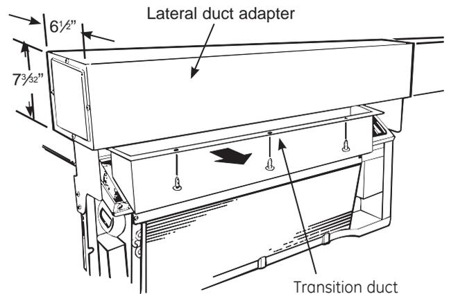
4. The old transition duct, the three screws (if used) and any gaskets used to seal the old transition duct to the chassis will not be needed for the new installation but should be kept for possible reuse of the old chassis in this installation location.
