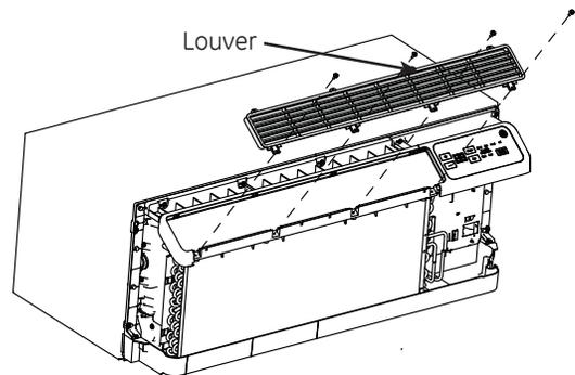
4. Align the metal seal strip as shown and secure with the four louver mounting screws.
