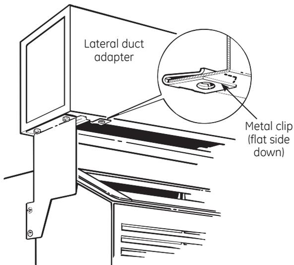
3. Remove the transition duct and drill two 1/4" diameter holes at the center punch locations. Slide the metal clips onto the flanges at these holes as shown in the illustration.
