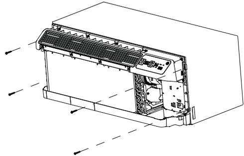
3. Remove and save the four screws securing the louver to the chassis. Lift up and remove louver.
