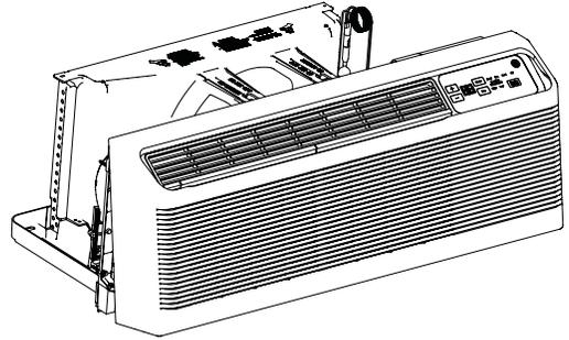
2. Slide the chassis into the case and secure with the four screws supplied with the Zoneline unit through the chassis flange holes.
