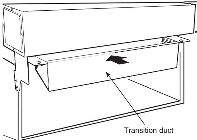
2. Center punch the transition duct mounting screw hole locations into the lateral duct adapter. Use the holes in the flanges at each end of the transition duct as a template. Make sure that the transition duct is all the way back when the center punch impressions are made.
