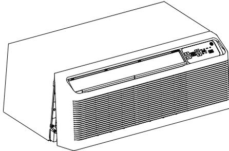
7. Remove the air filters from room cabinet front.
